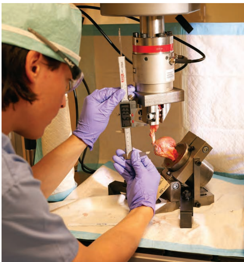
The biomechanical tests were performed in real-time using the Instron ElectroPuls E1000, allowing researchers to visibly see how well each surgical technique performed during testing procedures.
